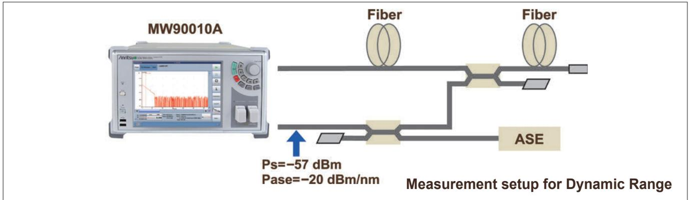
\*1: Ps: Maximum backscatter level at the input [dBm]
