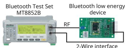
For EUT transmitter tests, test controls sent from the MT8852B configure the Bluetooth low energy device to transmit test reference packets that are captured and analyzed by the MT8852B receiver. The MT8852B-027/034/035/036 options are supplied with a Bluetooth low energy measurement application. During the design verification stages this application can be used to display the reference test packets transmitted by the EUT.
