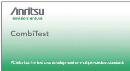
CombiTest is a software application used to remotely control Anritsu Bluetooth test sets using a user-configured test plan of measurements. It is ideal for creating design-verification or production test plans for Bluetooth radios. CombiTest allows users to install plug-ins as required for each test instrument.
