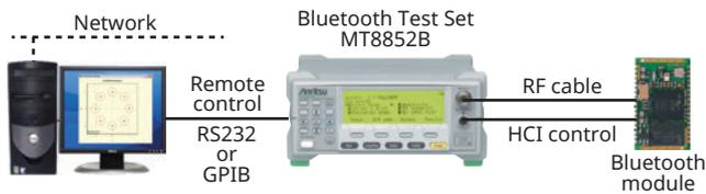
For fault finding and analysis, BlueSuite Pro3 software is a PC based tool kit that tests EUTs systematically on all channels. BlueSuite Pro3 also graphically displays the essential waveforms of power burst profile, modulation deviation and IQ diagrams. In the early stages of development, the signal generator and transmitter analyzer can be used to test the device without forming any protocol connection to the test set.
