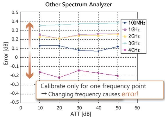
The absolute amplitude accuracy specifications of other spectrum analyzers excludes:
