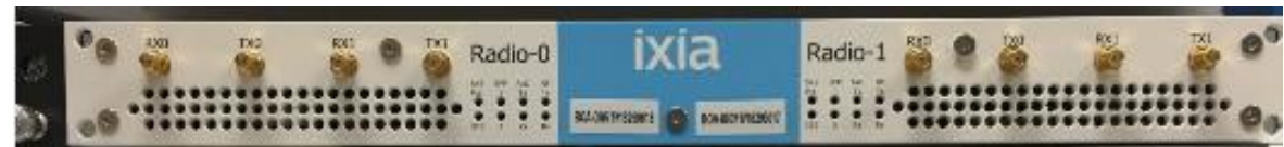
Radio Head (CPRI to Radio conversion)
