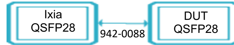
#2 2x50GE point-to-point Passive Copper DAC
