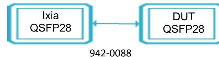
#2 1x40GE point-to-point Direct Attach Cable DAC
